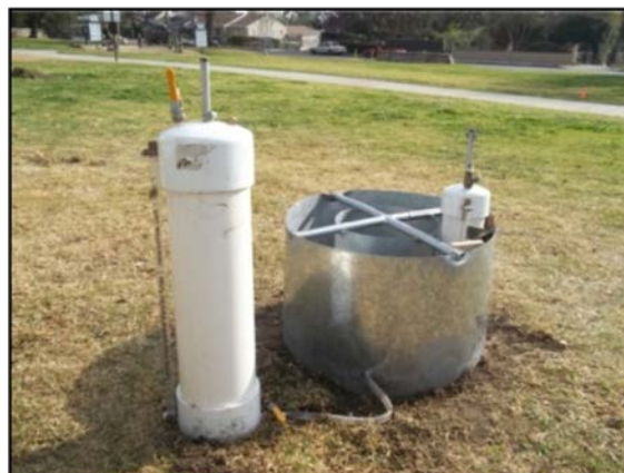
Double Ring Infiltrometer (ASTM D3385) Test Setup
