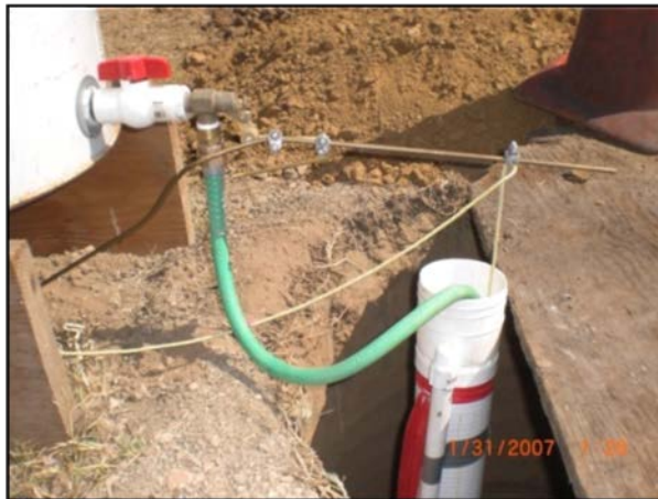
Well Permeameter (USBR 7300-89) Test Setup
